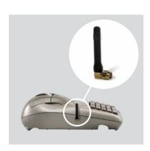
**GPRS** version Antenna for GPRS Modem
